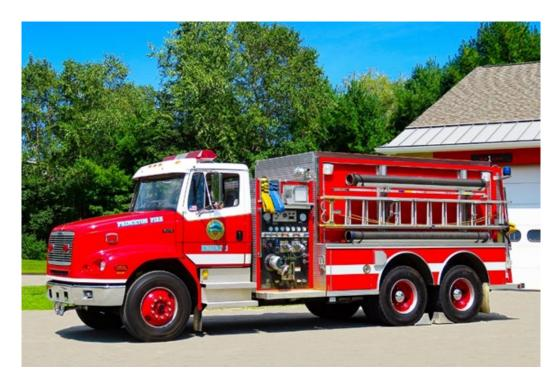
FIGURE IX-2 PRINCETON ENGINE 1: 1998 Central States tanker / pumper 1250 GPM pump capacity; 2500-gallon water tank
