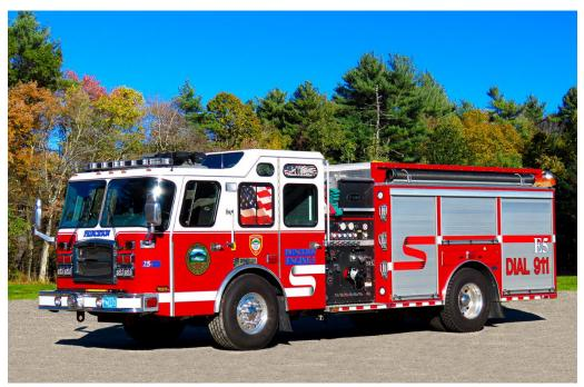
FIGURE IX-6 PRINCETON ENGINE 5: 2010 E-One Typhoon pumper 1500 GPM pump capacity; 1000-gallon water tank
