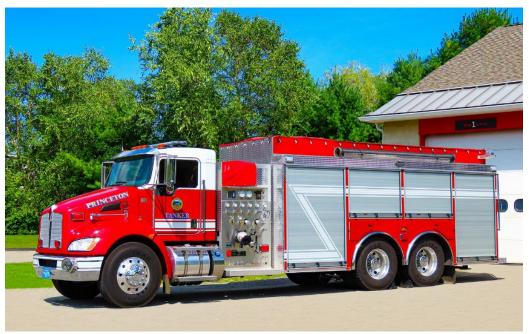
FIGURE IX-8 PRINCETON TANKER 1: 2018 Kenworth Deep South tanker 1500 GPM pump capacity; 2500-gallon water tank
