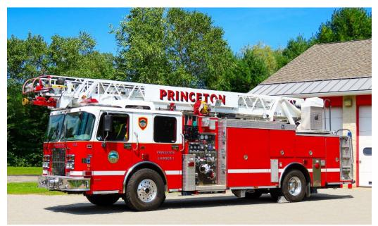
Figure IX-7 PRINCETON LADDER 1: 2006 Spartan/Smeal quint 75-foot ladder; 1500 GPM pump capacity; 440- gallon water tank
