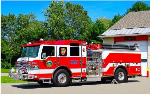
FIGURE IX-3 PRINCETON ENGINE 2: 2011 Pierce pumper 1750 GPM pump capacity; 1000-gallon water tank
